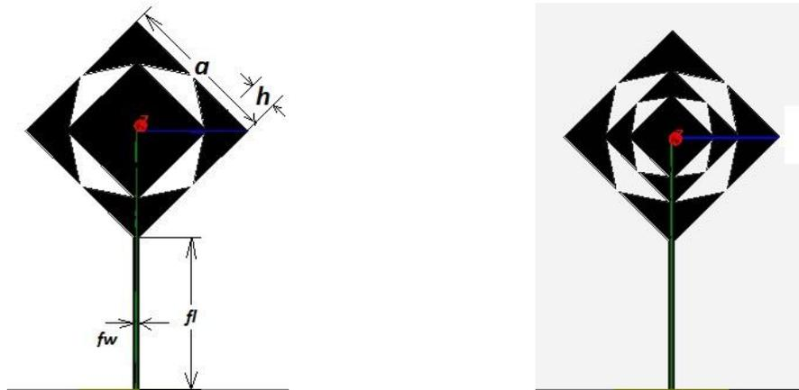
Figure 4. Simulated patch shape for basic antenna and next iteration fractal.
