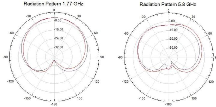
Figure 7. Radiation patterns for the basic antenna
