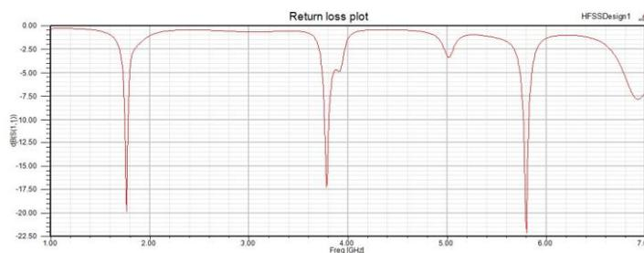
Figure 5. Simulated return loss for basic antenna
