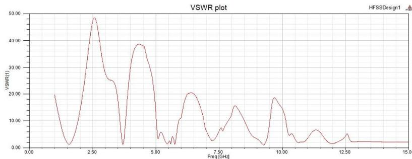
Figure 10. VSWR plot for the next iteration antenna
