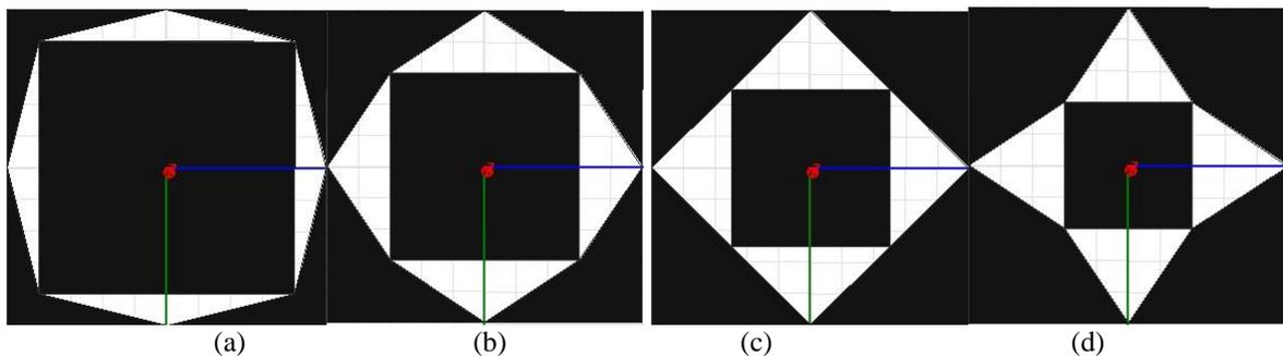
Figure 3. Geometry variations for different values of 'rt': (a)  $rt=0.1$  (b)  $rt=0.2$  (c)  $rt=0.25$  (d)  $rt=0.3$
